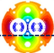
$BdL = 119.2 \text{ Tm} @ I_{\text{nom}} = 11.85 \text{ kA}$
