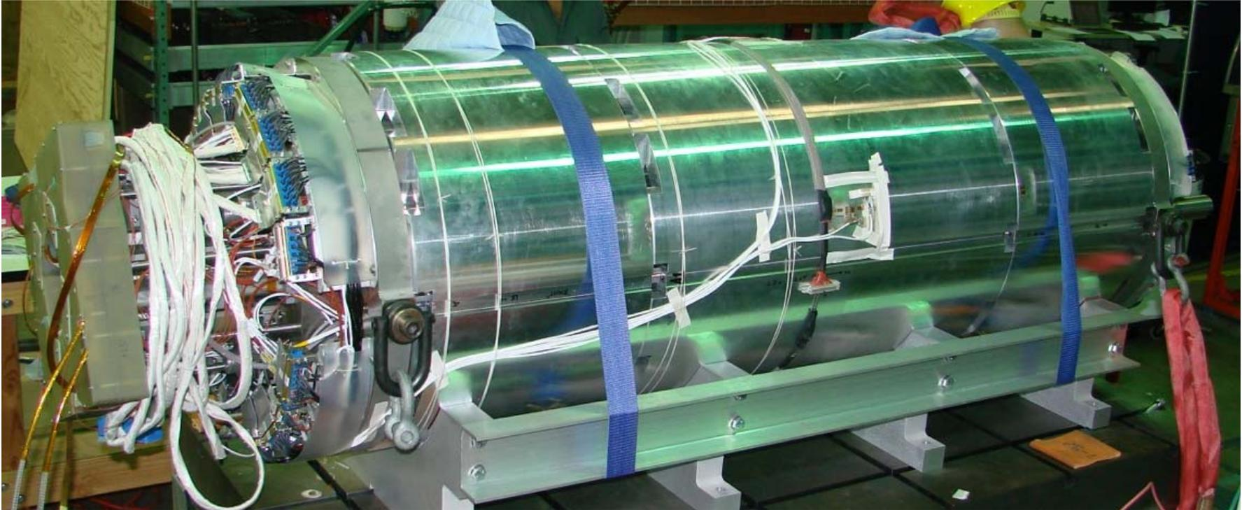
Test at FNAL in progress. The magnet tested at Fermilab consists of two coils manufactured at CERN and two others manufactured by the LARP (LHC Accelerator Research Program) consortium
