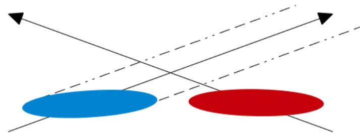
Bunches colliding with a crossing angle without (left) and with (right) the crab crossing
